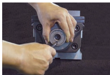
How to adjust the clamping force
